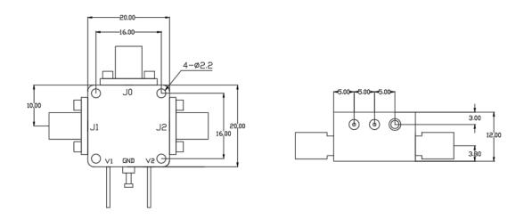
In millimetres with 1.85mm female connector
